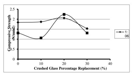
Figure 4: Graph showing strength of sandcrete hollow block with mix 1:6 and 1:8 cured with MgSO4 at 14 days
