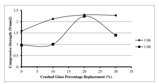
Figure 3: Graph showing strength of sandcrete hollow block with mix 1:6 and 1:8 cured with MgSO4 at 7 days
