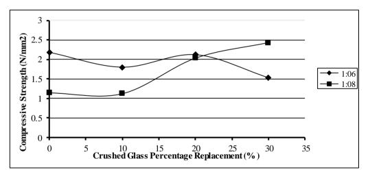
Figure 2: Graph showing strength of sandcrete hollow block with mix 1:6 and 1:8 cured with water for 14 days
