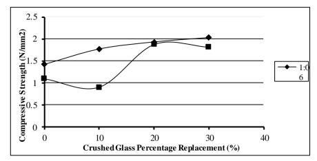
Figures 1 - 4 show the graphical representation of compressive strengths of the glasscrete block specimens.
